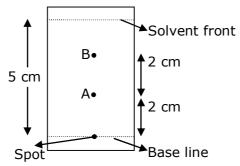
Fig: Paper chromatography for compounds A and B the calculated  $R_f$  value of A \_\_\_\_\_  $\times ~10^{-1}.$
